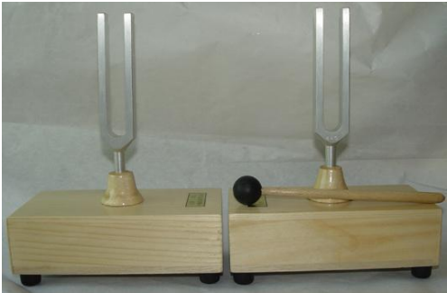
Beat frequency experiment on tuning fork
